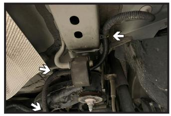
Using a flat screwdriver, unclip the electrical wire loom from the side of the frame and bottom of the vehicle to allow for receiver hitch installation. Do this on both sides of the vehicle.
