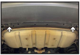
If present, using a flat screwdriver, remove the two (2) push pins from the rear underbody panel. Remove panel, it will not be reinstalled
