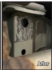
Using a flat screwdriver scrape the tape residue from the bottom and sides of the frame around the access and bolt holes.
